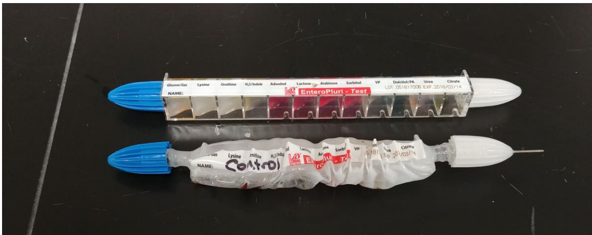
Figure 7. Un-autoclaved enterotube (top) and autoclaved enterotube (bottom). The enterotube innoculating needle protrudes from the media holder after autoclaving resulting in a sharps hazard.
